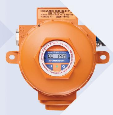
Lowering the cost of installation, the 4-wire addressable implementation drastically reduces cabling requirements. The large OLED display allows users to easily work with Xgard Bright during install, calibration and routine maintenance without the need to open the housing.
